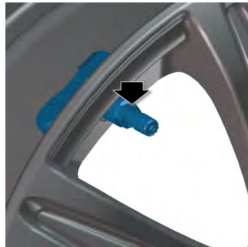
Remove the tire pressure sensor.
