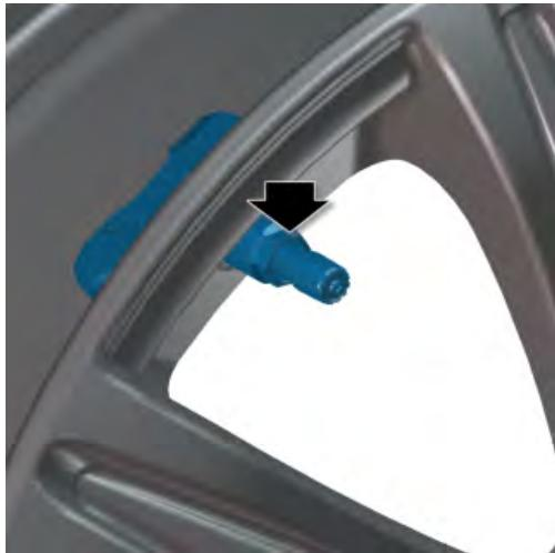
Install the tire pressure sensor. Torque the nut to 8 Nm.
